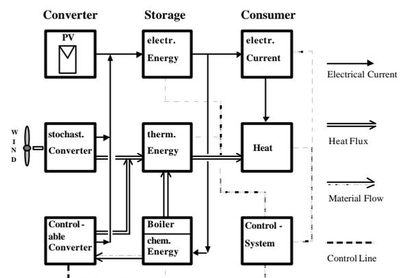
**Figure 1:** Principle Scheme of a Hybrid System
