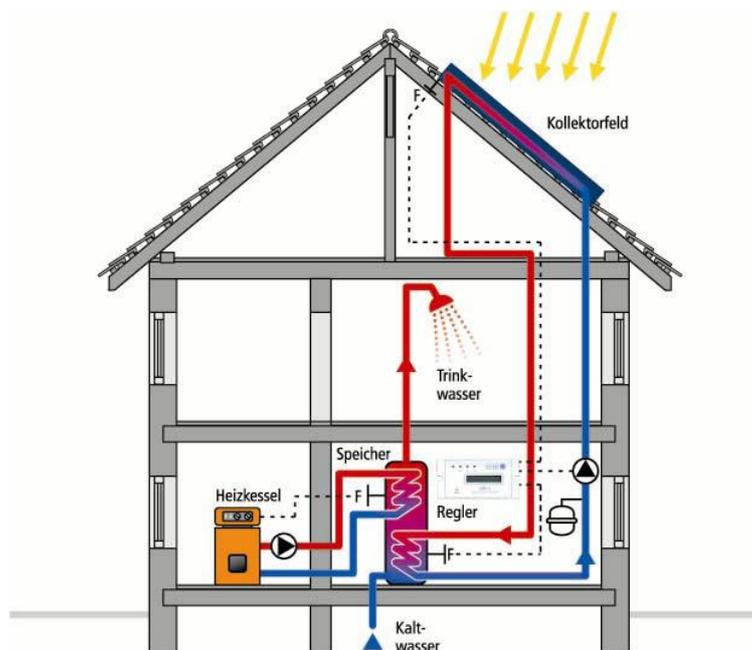
Figure 1: A solar thermal energy plant (DGS)
