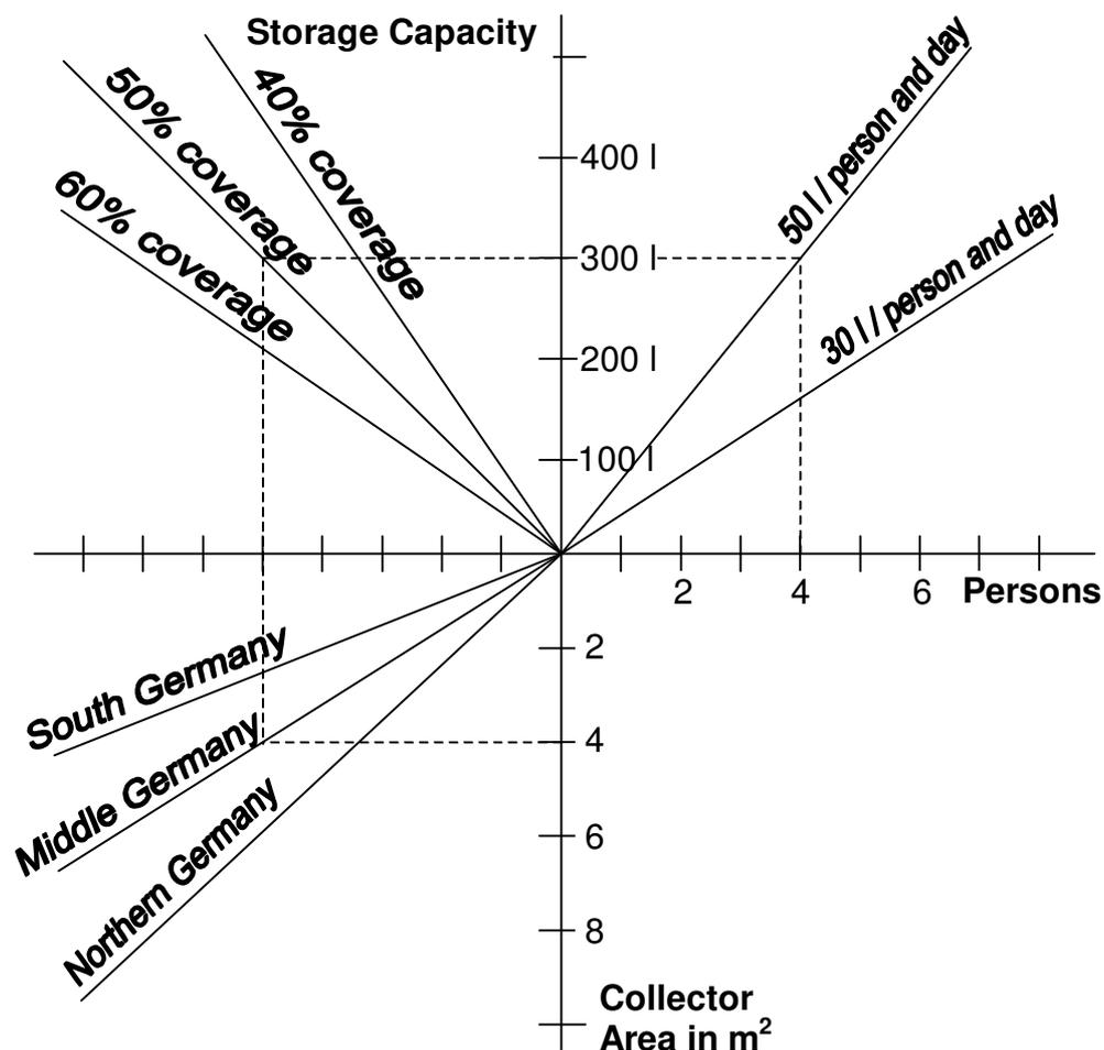
Figure 3: Dimensioning Diagram
