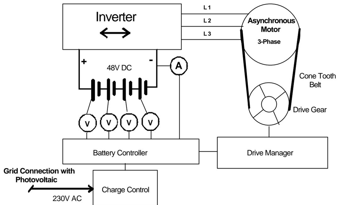
Figure 6: Driving system concept for electric vehicles
