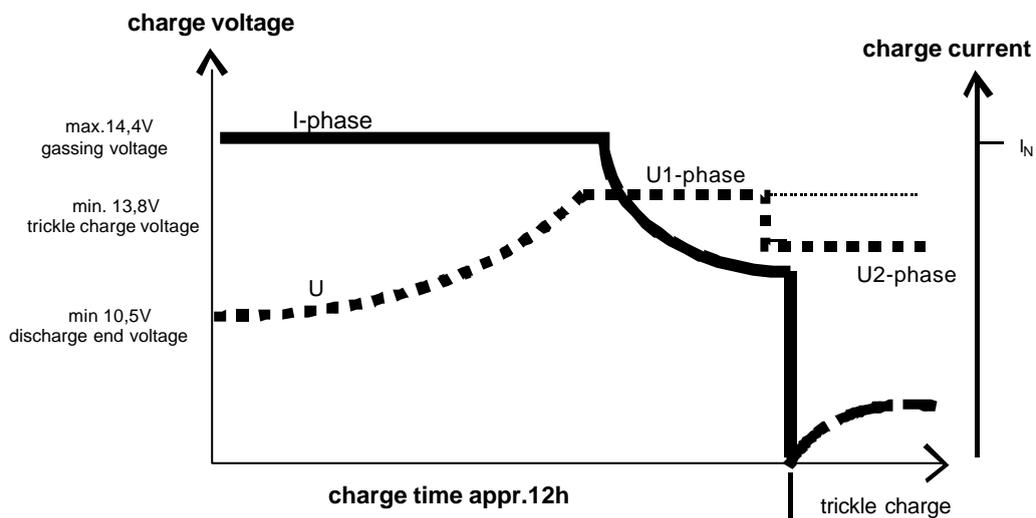
Figure 3: Principal charge characteristics of a lead-jelly battery
