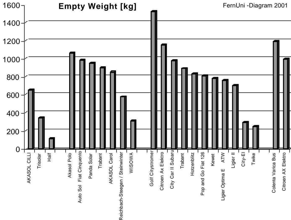
Figure 5: Empty weight of electric vehicles at the Tour de Ruhr
