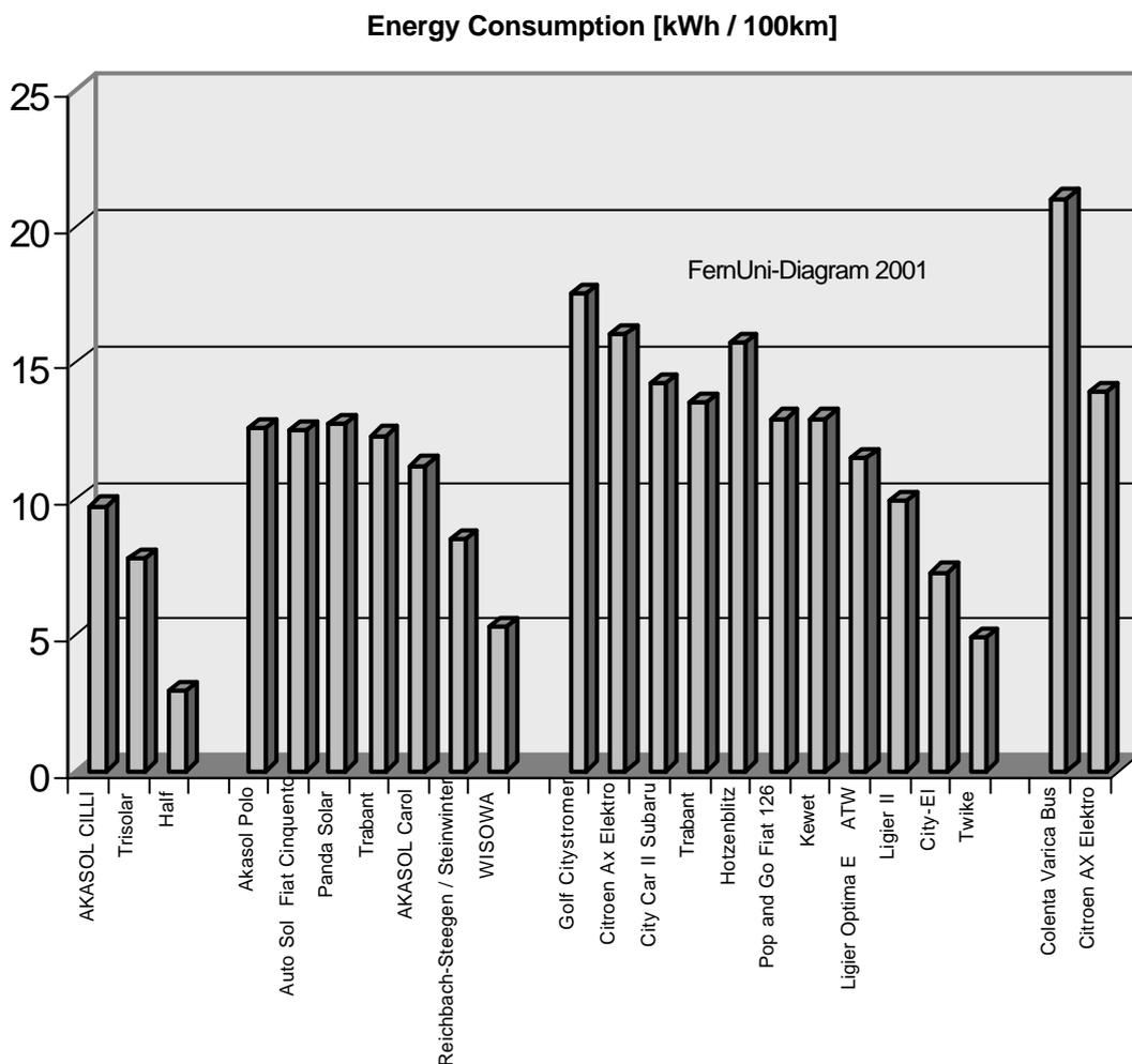
Figure 4: Average energy consumption of some electric vehicles for 100 km at the Tour de Ruhr
