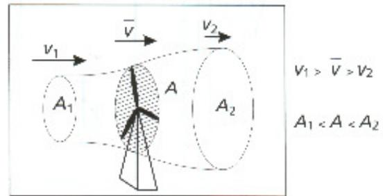
**Figure 2:** Wind Flow through the Rotor Area
