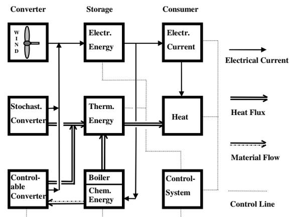
**Figure 1:** Fundamental Systematic of Hybrid Systems
