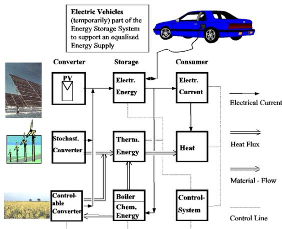
**Figure 2:** Electric Vehicle as a Part of the Electrical Storage System
