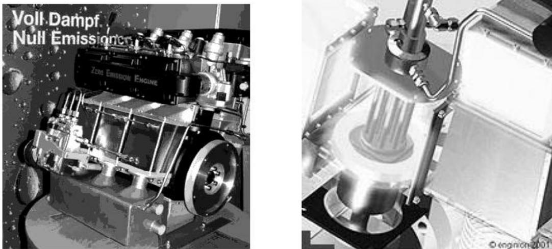
Figure 3: ZEE 03 with super heater [4], [5]
