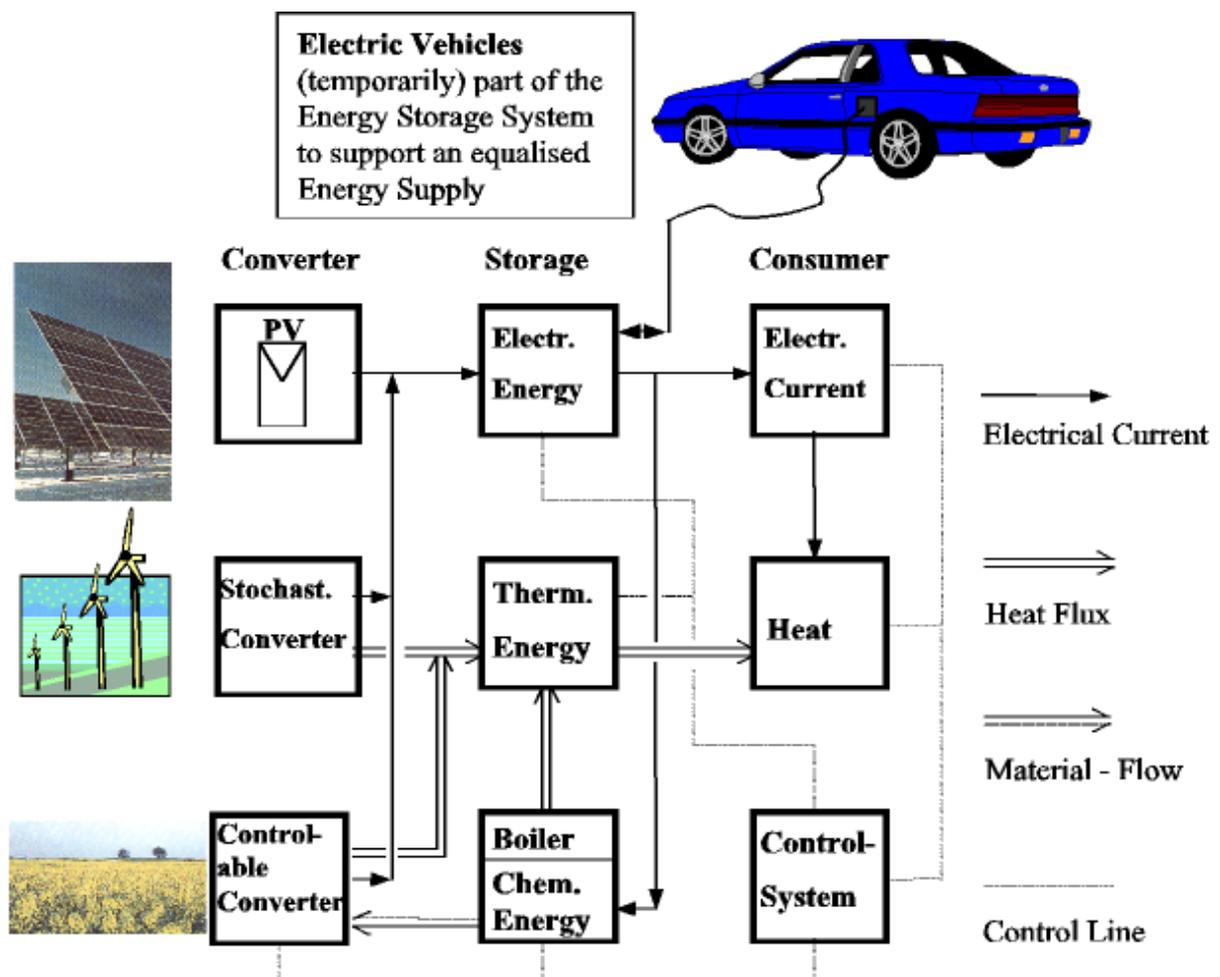
Figure 1: Structure of hybrid systems with electric vehicles [1], [5]
