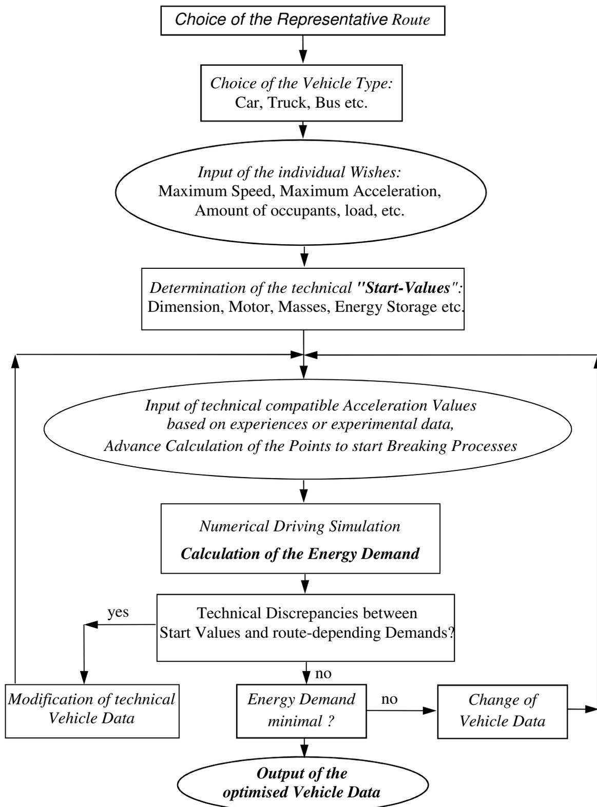
Figure 2: Process Scheme of the Optimisation Procedure [2], [3]
