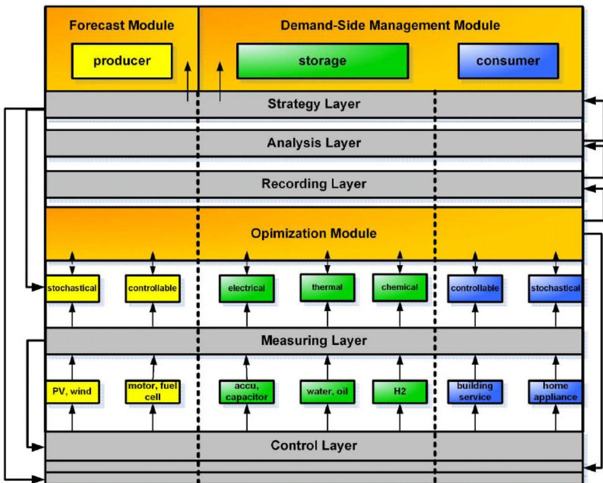
Figure 3: Layout of the EMS-Design [3], [8]
