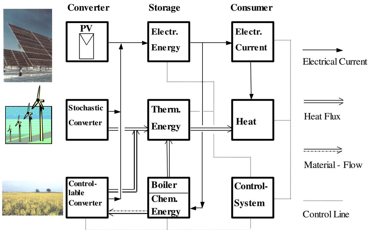
Figure 1 Fundamental Systematic of PV-Hybrid Systems
