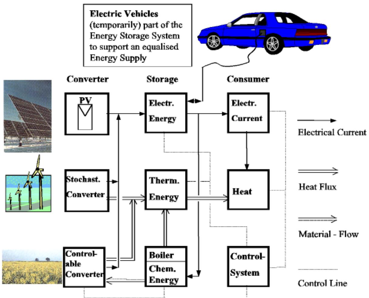
Figure 1: Structure of hybrid systems with electric vehicles [1], [2]
